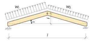
Figure 8.2 Three-pin truss with simple roof beams and tension member. Upward load.
