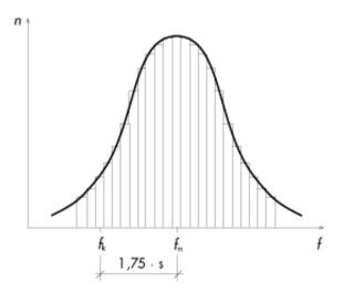
Figure 1.8. Example of a frequency diagram with superimposed normal distribution curve.
