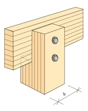
Figure 13.22 Pinned connection between beam and column with the beam recessed in the top of the column. Principles.
