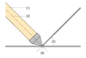
Figure 2.16. System lines should if possible meet at one point, to avoid moments in the node. (1) strut. 2) System line. (3) tie. (4) Theoretical node.
