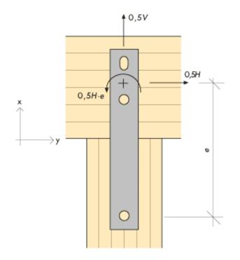
Figure 13.20.The fishplate is regarded as a beam rigidly fixed at one end and freely supported at the other. Symbols.
