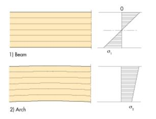
Figure 2.10 Bending stresses in a loaded beam (1) vary through the depth. Compression at the top and tension at the bottom. At the centre of the cros section the stress = 0. An arch (2) on the other hand has compression throughout its cross-section.
