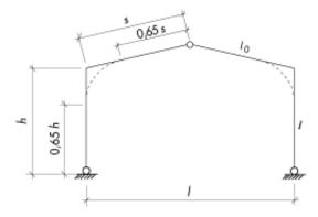
Figure 9.3. Fictitious buckling length for frames. Symbols.
