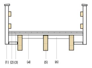
Figure 16.6 Girder bridge with transverse secondary beams and planks. (1) Handrail. (2) Road surface. (3) Planks. (4) Transverse secondary beam. (5) Glulam beams. (6) Wind bracing.
