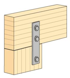
Figure 13.18 Pinned connection between beam and column with fishplates of flat steel. Principles.
