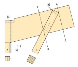
Figure 9.9 Built-up haunch with bolted connection between rafter and inner leg.
