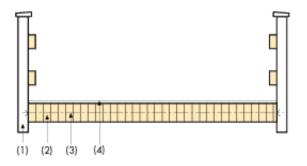
Figure 16.4 Slab bridge with transversely pre-stressed slab of glulam. (1) Handrail. (2) Upright glulam beams. (3) Steel tension rod. (4) Road surface.
