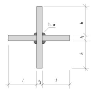
Figure 13.28 Cruciform connector of welded flat steel for transfer of shear forces.
