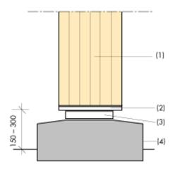
Figure 1.12. Design for timber protection. Example. 1) Glulam column. 2) Moisture barrier, i.e. oil treated hard board. 3) Bearing plate of steel. 4) Concrete foundation.
