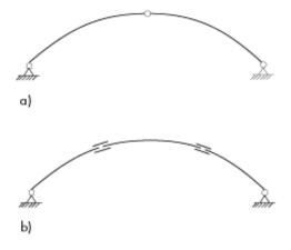
Figure 10.3 Suitable placing of joints in arch structures. a) Hinge b) Rigid joint.
