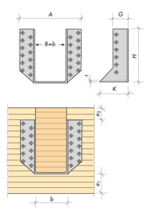
Figure 14.8. Connection of secondary beam using BMF hanger: R30.
