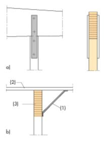
Figure 4.1 Lateral restraint at intermediate support. a) with U-section or heavy fishplate. b) with diagonal bracing. (1) from purlin (2) to bottom edge of beam.
