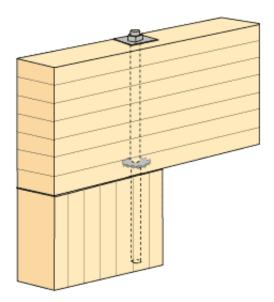
Figure 13.21 Pinned connection between beam and column with glued-in bolt. Principles.
