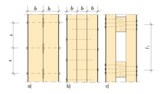
Figure 5.4 Section through mechanically jointed column. a) Continuously bolted. b) Continuously nailed. c) With spacers.
