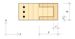
Figure 13.14 Rigidly fixed column base with glued-in bolts and steel base. Calculation model.
