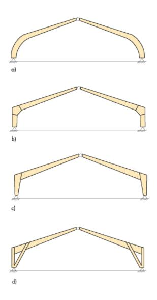
Figure 9.1 Examples of designs of three-pin portal frames a) Frame with curved haunches
