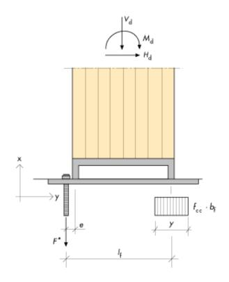
Figure 13.17 Rigidly fixed column base with glued-in bolts and steel base. Calculation model.
