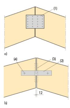
Figure 14.14 Ridge joint a) Nailplates (1): fire protection must be applied. b) BMF-type ridge fixture (3) steel flat (2) bolt (4) R30
