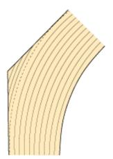
Figure 9.4. Curved haunch with fully glued corner piece.
