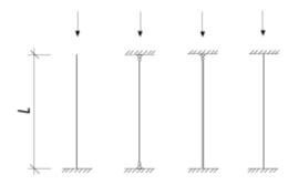
Figure 5.1 Various end conditions in buckling
