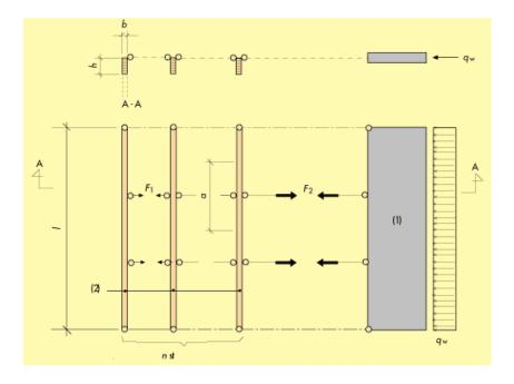
Figure 12.4. Lateral bracing of roof beams. 1) Laterally bracing structure. 2) Laterally bracing roof beams.
