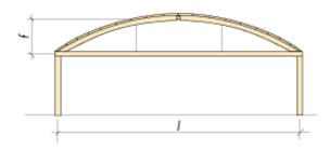
Figure 10.1 Arch with tie rod, on columns.
