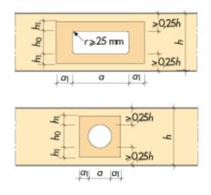
Figure 4.13. Plywood reinforcement of hole. Symbols.
