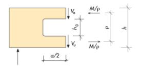
Figure 4.12 When designing rectangular holes it is necessary to take into account the effect of the moment caused by the shear force.
