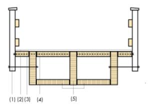
Figure 16.8 Pre-stressed box beam bridge. (1) Handrail. (2) Road surface. (3) Pre-stressed roadway. (4) Steel tension rods.
