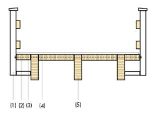
Figure 16.7 T-beam bridge with pre-stressed slab. (1) Handrail. (2) Road surface. (3) Pre-stressed roadway. (4) Steel tension rods. (5) Glulam beams.
