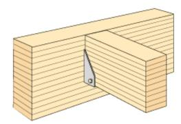
Figure 13.37. Pinned connection between secondary and primary beam with welded hanger. Principle.
