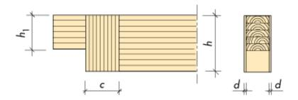
Figure 4.8 Notch in beam end. Plywood reinforcement .
