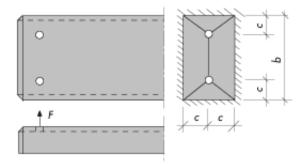
Figure 13.16 Steel base. Calculation model.
