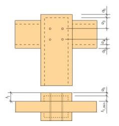
Figure 14.2. Increased sizes of unprotected joints for fire classes higher than R15.
