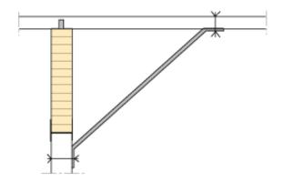
Figure 13.24 Side bracing of column top.
