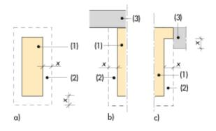
Figure 14.1 Effective residual section after fire (1) original section (2) To the left: Four sided fire exposure. Centre and to the right: Three sidedfire exposure, where the top is protected by material with better fire resistance (3).
