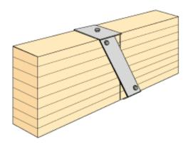
Figure 13.32 Pinned beam joint with Gerber fixture. Principle.
