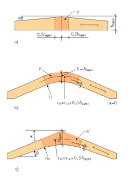
Figure 6.7. Curved beams with constant and varying depths. The characteristic volume V is marked in the figure.
