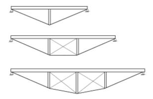
Figure 16.9 Examples of trussed systems with steel tension chord and timber posts acting as intermediate elastic supports.
