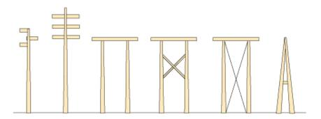
Figure 15.1 Examples of common types of glulam poles.
