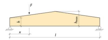
Figure 6.6 Simply supported, double tapered beam with concentrated load.
