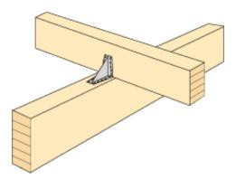
Figure 13.36 Fixing purlins with angle of cold-formed steel.
