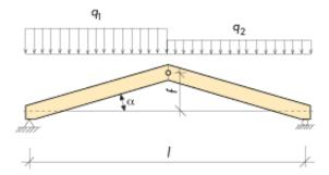
Figure 8.1 Three-pin truss with simple roof beams and tension member. Downward load.
