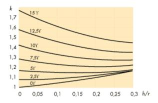
Figur 6.8 Coefficient  $k_i$  for curved beam with varying depth and with different roof slopes and curvature.
