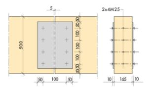
Figure 14.12 Bolted beam joint: R30.
