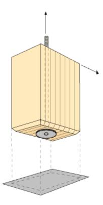
Figure 13.7 Pinned fixing of column base with glued-in bolt. Principle.
