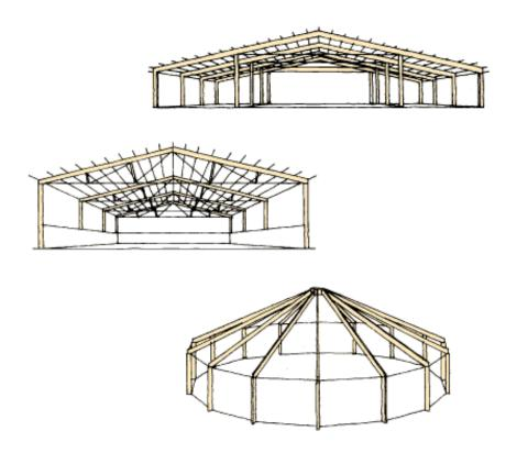
Figure 2.7 Three-pin trusses.
