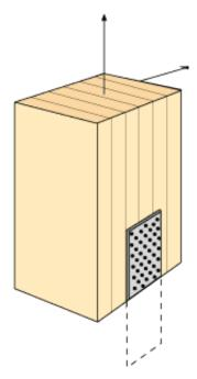
Figure 13.1 Pinned fixing of column foot with fishplates of nailplate. Principle sketch.
