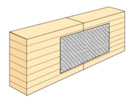
Figure 13.31. Pinned beam joint with fishplates of nailplate. Principles.
