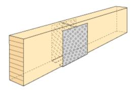
Figure 13.34 Gerber fixture type BMF-W.
