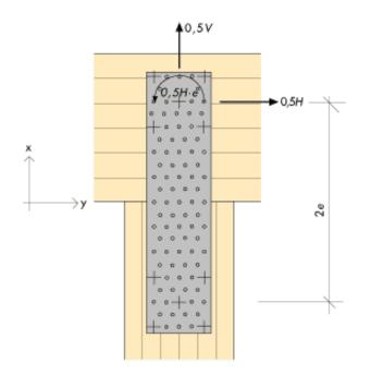
Figure 13.19. The fishplate is regarded as a beam rigidly fixed at both ends. Symbols.
