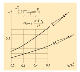
Figure 5.2 Diagram for determining the buckling load of columns whose cross-sectional depth has a linear variation.
