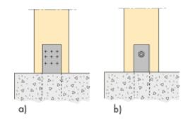
Figure 14.3 Pinned fixing of column base. a) Cast-in nailplate: R60. b) Cast-in flat steel and screw/bolt: R60.
