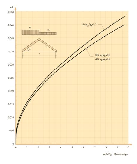
Figure 8.5 Diagram for design of three-pin truss regarding carrying capacity. The roof beams are assumed to be restrained from lateral buckling. Condition:  $f_{md}/f_{cd}$ = 1.1 and  $E_{md}/f_{cd}$ = 370
