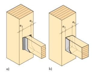
Figure 14.10. Edge distance at beam-column connection with BMF-type hanger: R30 under certain conditions (see table 14.2). a) Bent-out flaps. b )Bent-in flaps.
