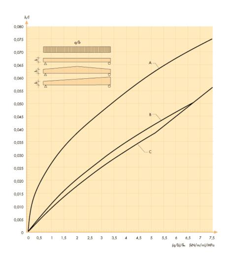
Figure 6.10 Diagram for design of beams supported at two points with regard to carrying capacity. Straight, double tapered and single tapered beams. The beams are assumed to be restrained against lateral buckling. Curve A = straight beam, Curve B = double tapered or single tapered beam 1:20, Curve C = double tapered or single tapered beam 1:16
