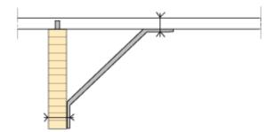
Figure 13.25 Bracing of continuous beam.
