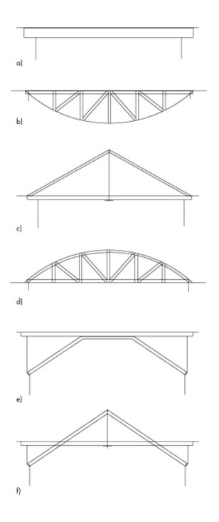
Figure 16.1 Girder Bridge types a) Simple girder. b) Bottom tensioned girder. c) King post. d) Truss. e) Strut frame. f) Combined king post-strut frame.
