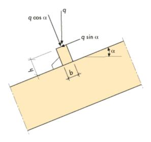
Figure 11.3 Vertical load on inclined purlin divided into components.
