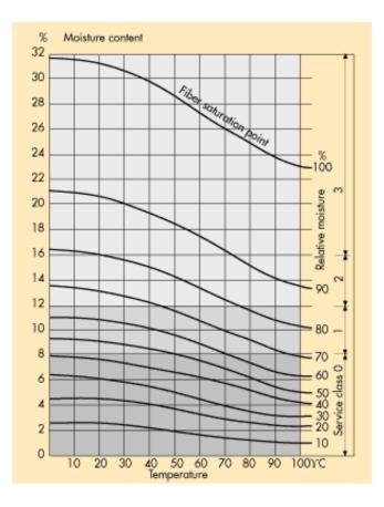
Figure 3.1 Equilibrium moisture content in timber as a function of the temperature at different levels of vapour pressure.
