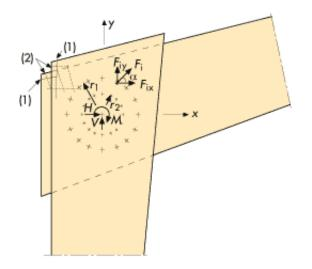
Figure 9.7 Bolted frame haunch. Symbols.
