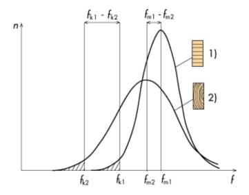
Figure 1.7. Structural components of glulam have higher average strength and a smaller spread of strength characteristics than corresponding components of structural timber.
