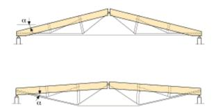
Figure 8.4 Three-pin truss with timber struts and steel ties.
