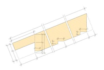
Figure 1.14. Example of dimensioning.
