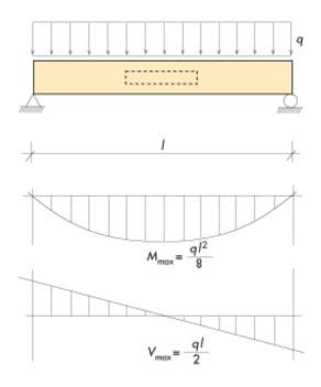
Figure 2.3 External moments and shear forces in a beam freely supported at two points with an evenly distributed load.
