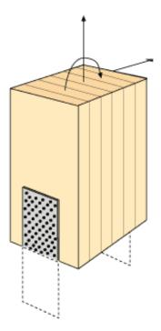
Figure 13.9. Rigidly fixed column base with fishplates of nail plate. Principle.
