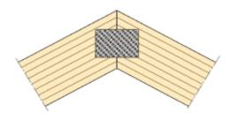
Figure 13.26 Pinned ridge joint with fishplates of nailplate. Principles.
