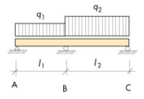
Figure 6.1. Continuous beam on three supports
