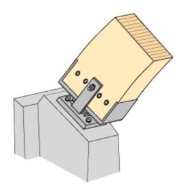
Figure 13.43 Welded support fixture with hinged connection. Principles.
