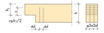
Figure 4.9 Notch in beam end. Reinforcement with glued-in screws.
