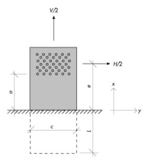
Figure 13.2. Nailplate as a rigidly fixed cantilever.
