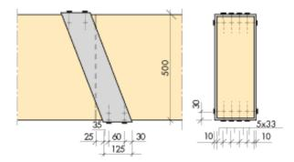
Figure 14.13. Beam joint with Gerber fixture: must be protected.
