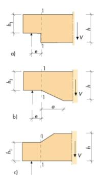
Figure 4.6. Notches in beam end. Symbols.
