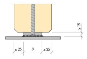
Figure 13.8 Fixing with end plate welded to fixing plate cast into the foundation.
