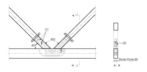
Figure 7.3 Example of design of node in a long-span truss
