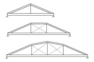
Figure 16.10 Examples of trussed systems with glulam compression chords and timber posts acting as intermediate elastic supports.
