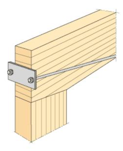
Figure 13.39 Fixing of steel tie. Principle.
