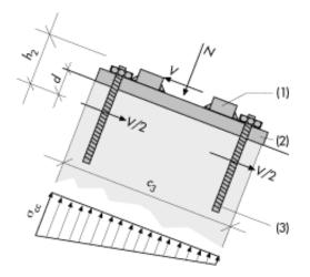
Figure 13.46 Transfer of forces between fixture and concrete. Calculation model. (1) Steel projection (2) Hinge plate (3) Anchor bolt
