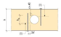
Figure 4.14 Reinforcement of hole using glued-in screw.
