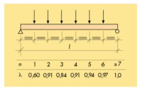
Table 4.2. Effective beam length *l*<sub>e</sub>in relation to total beam length. Simply supported beam, restrained from buckling at supports and loaded with n equal loads. The concentrated loads bear at the top edge of the beam and restrain lateral bending in the beam at the loading points.
