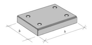
Figure 13.15 Steel base for rigidly fixed columns with glued-in bolts.
