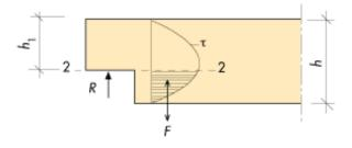
Figure 4.7 Reinforcement of notch in beam end. Symbols.
