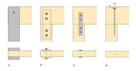
Figure 14.6. Connection between column and beam. a)Concrete fork: R60. b)Glulam fork: R30-R60. c)Steel flats: R30. d)Glued-in screw: R30-R60.
