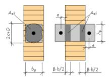
Figure 13.40. Effective contact area with one or two tie rods. Symbols.
