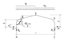
Figure 9.2 Three-pin frame with curved haunches. Symbols.
