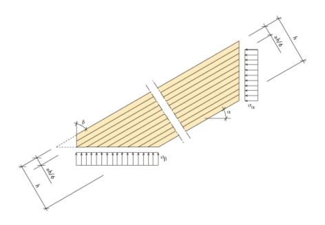
Figure 4.5. Contact pressure at sharp corners.
