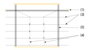
Figure 11.4 In steep roofs the other purlins can be hung up from the ridge purlin. (1) ridge purlin; (2) Other purlins; (3)Roof beam; (4) Suspension rod.
