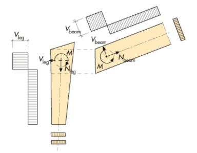
Figure 9.8 Cross-section forces and lateral force diagram for frame beam and frame leg.
