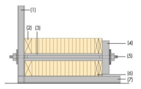
Figure 1.4. Schematic section through gluing bench. (1) Vertical stop. (2) Pressure distributing base, possible camber pattern. (3) Distance piece. (4) Compression block. (5) Tension screw. (6) Pressure distributing boards. (7) Horizontal stop.
