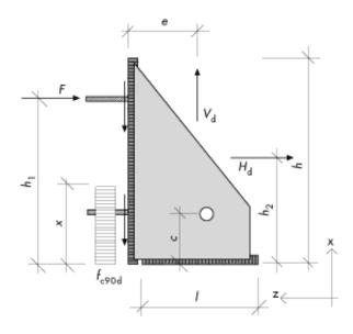
Figure 13.38 Welded beam hanger. Symbols.
