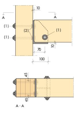
Figure 14.11. Beam connection with steel bracket and screws/bolts with connectosr: R30.
