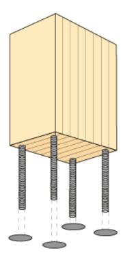
Figure 13.12 Rigidly fixed column base with glued-in bolt. Principles.
