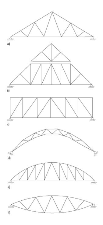
Figure 7.1 Types of truss. a)Triangular, b) Ditto, in parts for transport, c) Parallel, d) Two hinge arch, e) Bowstring, f) Fish belly
