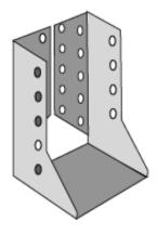
Figure 14.9 Hanger with bent-in flaps.
