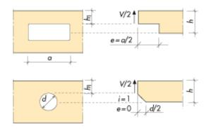
Figure 4.12 Analogy between holes and notches at the end of a beam. Symbols.
