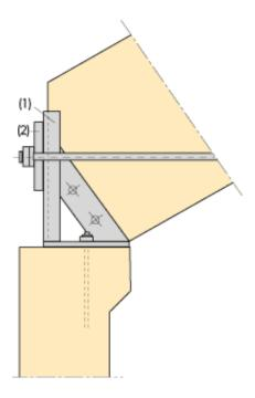
Figure 14.15 Steel tie fixture: fire protection must be applied. U-channel section (1), steel flat (2).
