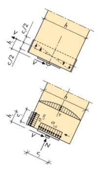
Figure 13.45. Transfer of forces between fixture and glulam. Calculation models.
