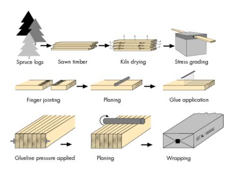
Figure 1.2 Glulam manufacture. Schematic.
