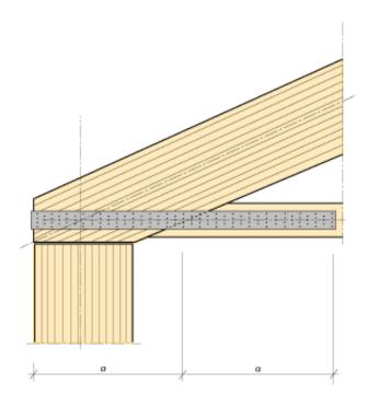
Figure 13.41 Fixing of glulam ties. Principles.
