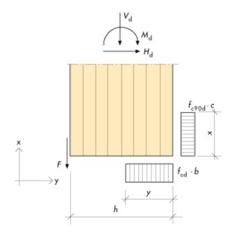
Figure 13.11. Rigid fixing with fishplates. Calculation model with compression stress blocks. Symbols.
