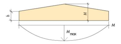
Figure 2.2. The shape of a symmetrical double pitched beam approximates to the moment diagram of a beam freely supported at each end. It is therefore more economic in material than a constant-depth beam.
