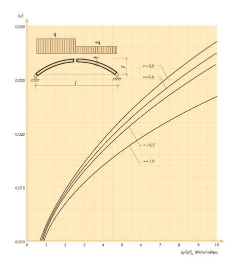
Figure 10.6 Diagram for design of 3-pin parabolic arch with reference to carrying capacity. The arch is assumed to be restrained from lateral buckling. Rise ratio of the arch f/I = 0,14.
