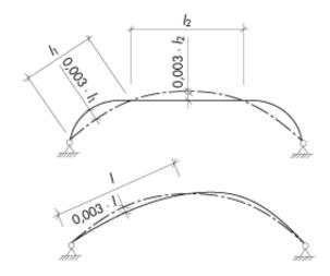
Figure 10.5 Example of an assumed initial deformation under symmetrical and unsymmetrical loadings. I, I1 and I2 are the distances between points which have not moved during the deformation of the arch.
