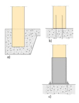
Figure 14.5 Rigidly fixed column base.a) Concrete column pocket: R60. b)Glued-in bolt: R30-R60. c)Steel column pocket: Must be fire protected.
