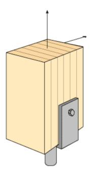
Figure 13.5 Pinned fixing of column foot using steel base shoe. Principle sketch.
