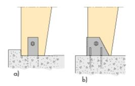
Figure 14.4 Pinned fixing of frame base. a) With concrete projection: R60. b) Steel shoe: R30.
