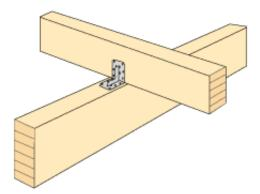
Figure 13.35 Fixing purlins with stiffened angle fixture of cold-formed steel plate.
