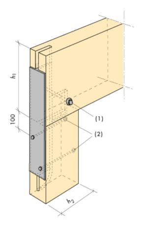
Figure 14.7. Connection column-beam with slotted-in T-section: R30-R60.
