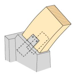
Figure 13.42 Springing point of arch with flat steel and screws/bolts. Principles.
