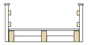
Figure 16.5 Girder bridge with planks laid direct on the glulam beams.
