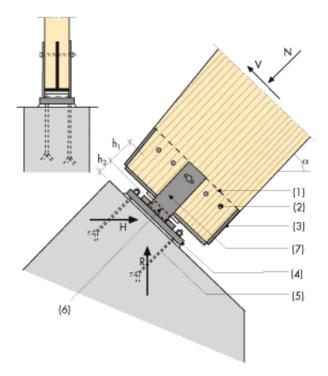
Figure 13.44 Symbols. (1) ^ section, welded or cut I beam. (2) Steel dowels and/or screw/bolt. (3) End plate. (4) Lower hinge plate with steel projections. (5) Anchor bolts. (6) Upper hinge plate with steel projections. (7) Side plates (NB: elongated screw/bolt holes).
