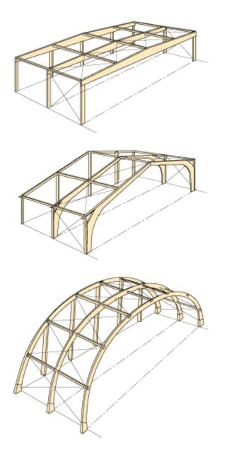
Figure 12.3 Wind bracing of frame and arch structures.
